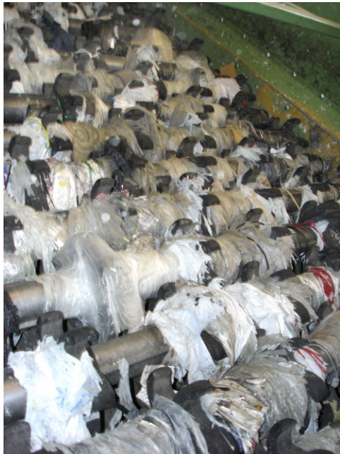
Screen at the Boulder County Recycling Center clogged with plastic bags.
