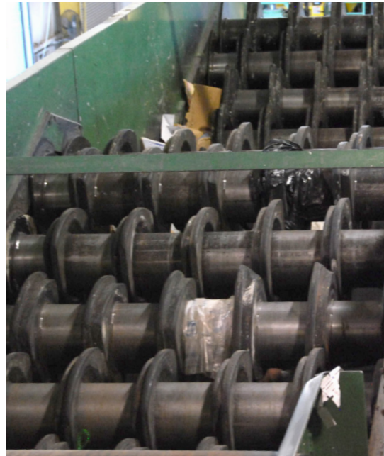
An unlogged screen after many hours of hand-cleaning.
